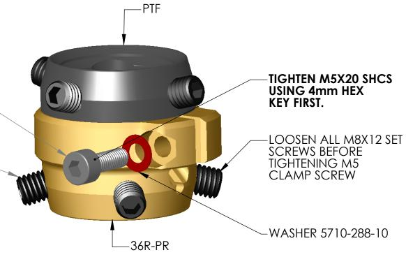
Critical Tips on Bolt and Screw Installation
